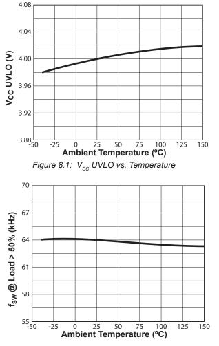
Figure 8.3: Switching Frequency vs. Temperature <sup>1</sup>
