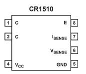
Figure 4.1: 7-Lead SOIC Package
